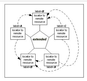
This diagram reflects directional traversal arcs created by the following settings, where both As and Cs are allowed to initiate traversal to all Bs. Because some labels appear on several resources, each arc specification potentially creates several traversal arcs at once:
