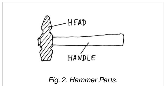
Fig. 2. Hammer Parts.
